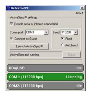
On starting, DetectoidPC will check for the availability of COM ports, as well as IrDA/USB support. Once the terminal is detected, the port status will change from Idle to Listening as shown in the screen shot above.
