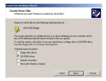
In the "Locate Drive Files" dialog, check the CD-ROM drives check box and insert the driver CD provided into the CD tray on your PC. There are sub-directories in this directory for each type of Windows OS supported. Select stirusb.sys file in the correct sub-directory for your PC:
