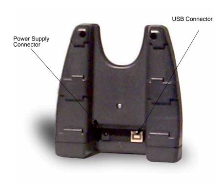
There is a 5V DC power supply connector and a USB connector:
