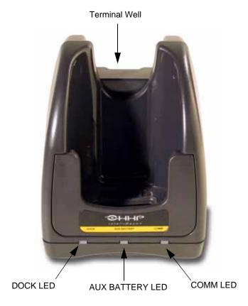
**Dolphin Terminal Well** Place the Dolphin in this well to communicate with a host device and to charge the Dolphin's battery. **LEDs** There are three LEDs on the front panel of the IntelliBase+:
