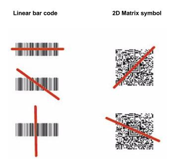
The aiming beam is smaller when the terminal is held closer to the code and larger when it is farther from the code. Symbologies with smaller bars or elements (mil size) should be read closer to the unit. Symbologies with larger bars or elements (mil size) should be read farther from the unit.
