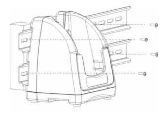
In either case, **after wall mounting**, it is **recommended** that the cables be secured to the DIN rail through use of a wire tie to prevent damage to the IntelliBase/USB HomeBase unit in case accidental or excessive force is applied to the cables.
