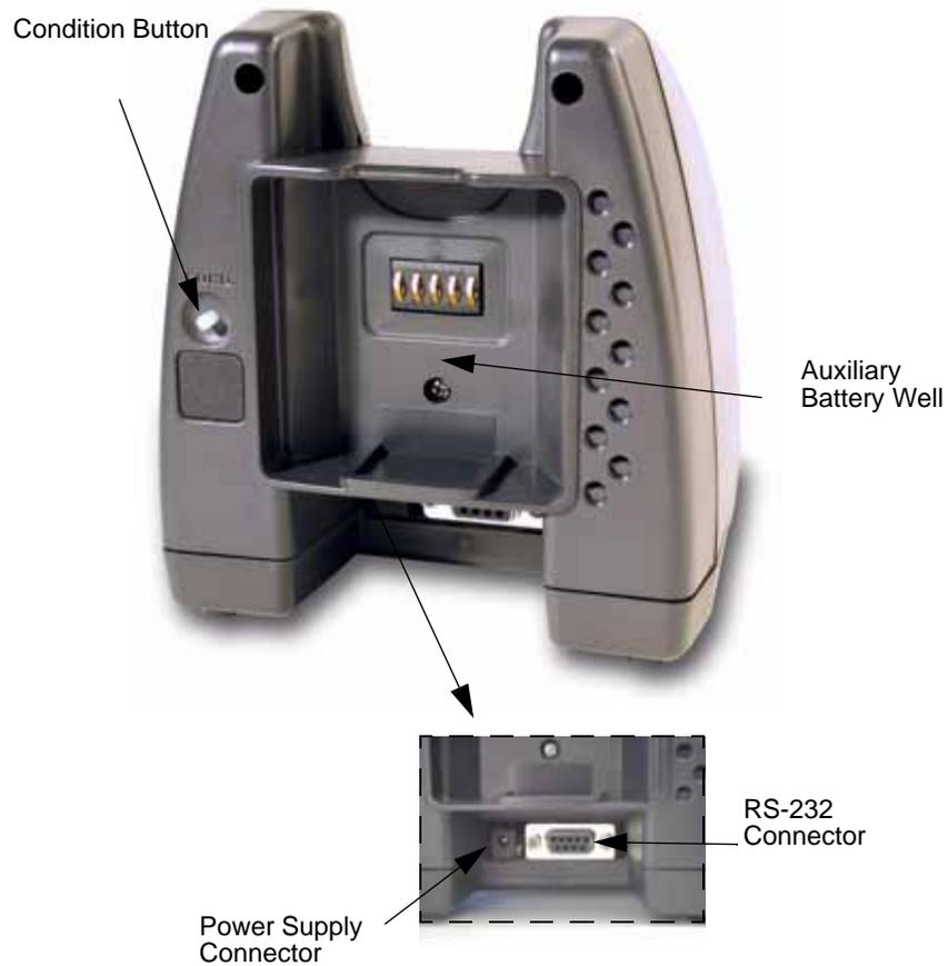
**Power supply connector** Use this connector to attach a power supply to the IntelliBase. The power supply provides 5V DC input for communications and battery charging.
