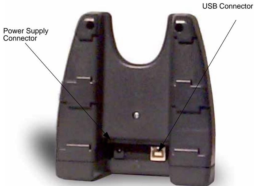
There is a 5V DC power supply connector and a USB connector:
