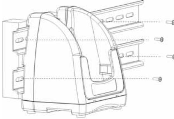
In either case, **after wall mounting**, it is **recommended** that the cables be secured to the DIN rail through use of a wire tie to prevent damage to the IntelliBase/USB HomeBase unit in case accidental or excessive force is applied to the cables.
