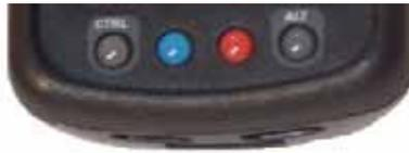
All three versions of the Dolphin 7400/7450 keyboard feature the standard PC keyboard modifier keys, **Alt**, **Ctl** and **Shift**. For single-handed operation, the **Shift** key only modifies the next key pressed; it must be pressed and released before each key you wish to modify. Functions of the Alt and Ctl keys are dependent on the software application in use.
