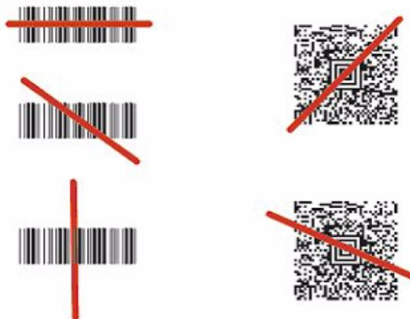
The aiming beam is smaller when the terminal is held closer to the code and larger when it is farther from the code. Symbologies with smaller bars or elements (mil size) should be read closer to the unit. Symbologies with larger bars or elements (mil size) should be read farther from the unit.
