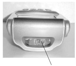
Reading aperture of bar code scanner
