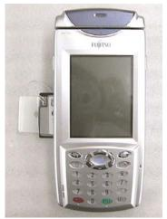
Insert card completely and tuck the pull-tab and antenna cables into the slot. Take off ABS resin block and rubber from side cover.
