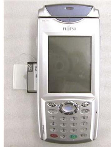
Insert card completely and tuck the pull-tab and antenna cables into the slot. Take off ABS resin block and rubber from side cover. Remove protective sheet of adhesive tape from card stopper and attach card stopper with side cover to the spot where the ABS resin block and rubber were attached. Attach side cover to main unit
