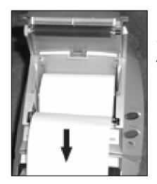
\*\*CAUTION: Do not manually force the paper through the printer mechanism. Doing so may cause damage to the printer unit.
