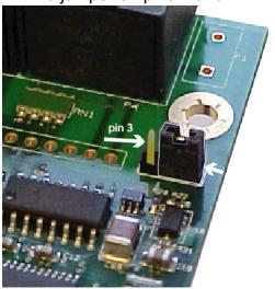
Note When the jumper is placed correctly for power in, the jumper will set on the pins closest to the edge of the board. The left arrow indicates the open pin and the right arrow is pointing to the jumper.
