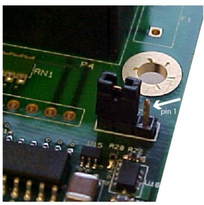
Note Here are the pins to verify the jumper position. The default position has the jumper on the two pins furthest from the edge. DO NOT MOVE THE JUMPER FROM THE DEFAULT UNLESS USING RI POWER
