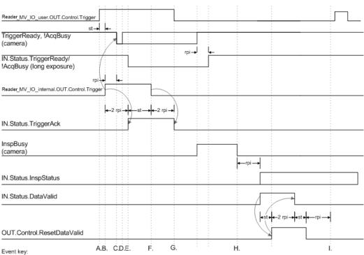
A. On rising edge of system trigger, the user app activates Reader\_MV\_IO\_user.OUT.Control.Trigger to trigger the demo code.
