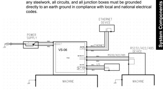
An earth ground is provided through the cable shields and chassis of the imager.
