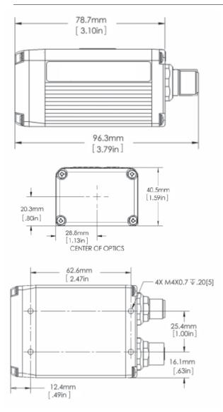
FIGURE C-1. VS-06 Smart Camera Dimensions
