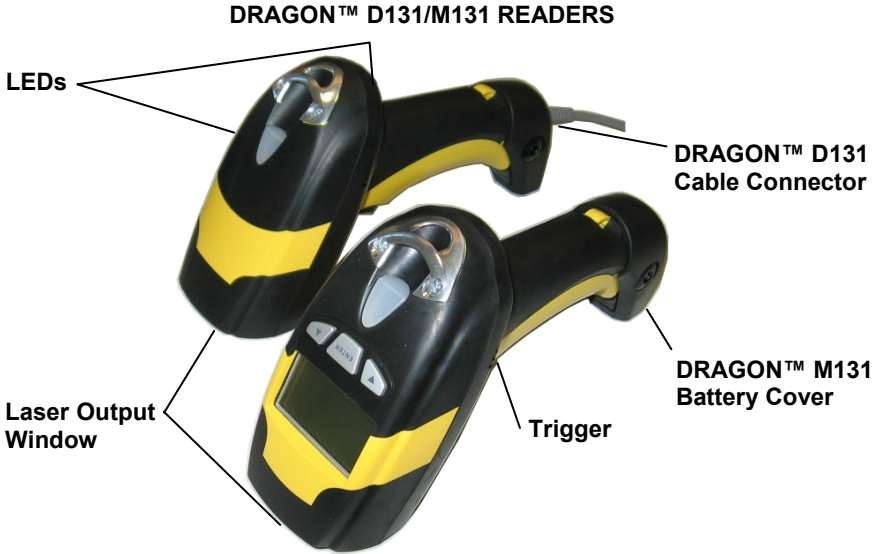
Figure A – DRAGON™ D131 and M131 Series Readers
