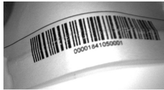
Figure 24 - Barcode Printed on Curved Surface Readable by Matrix 400™ in spite of Image Optical Distortion
