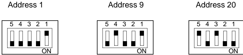
Figure 2.17 - DP1100 multidrop address selections
