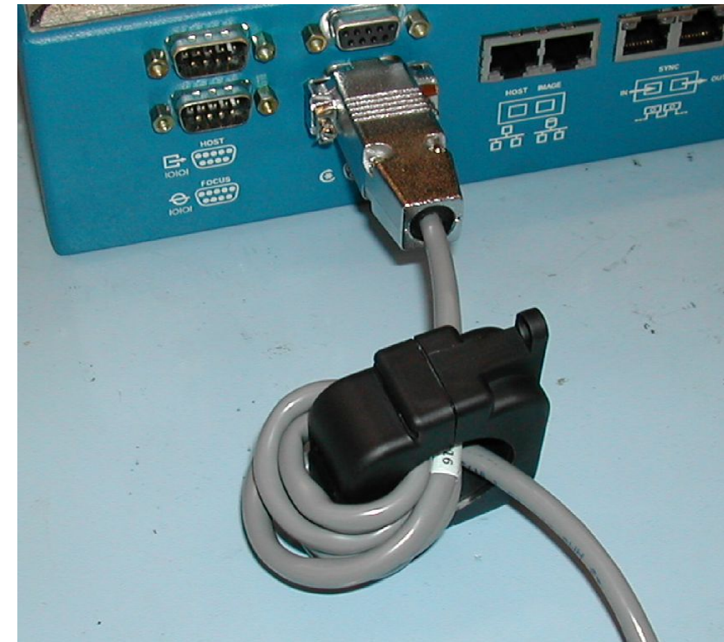
FERRITE INSTALLATION AND LOCATION SEE NOTE 3
