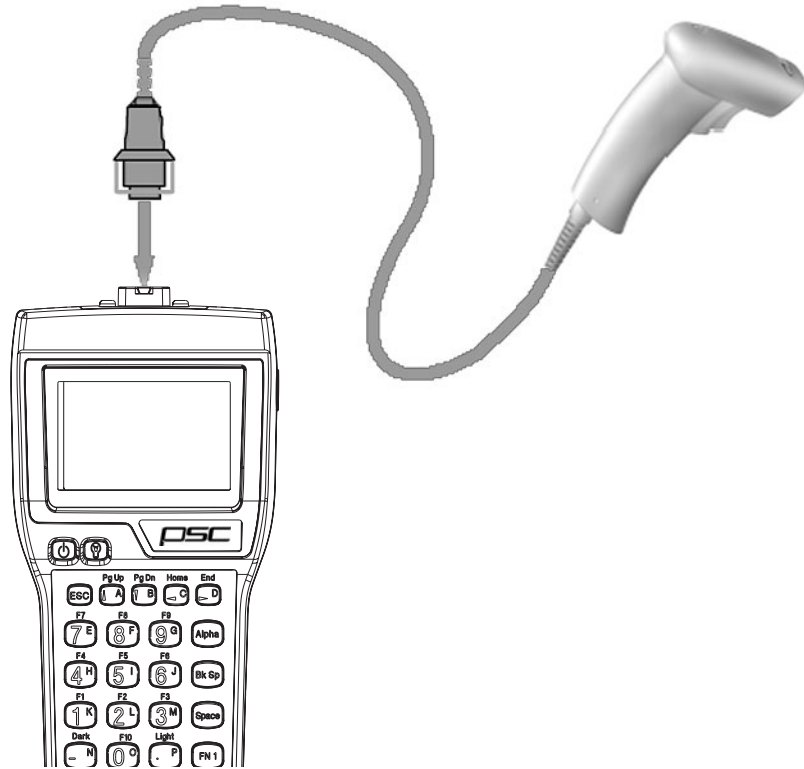
Figure 24. Attaching a PSC Snapshot to a Falcon 31x/32x
