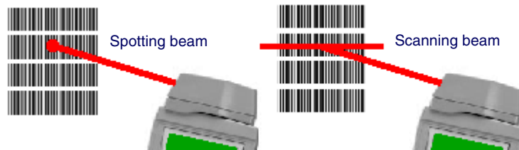
Figure 23. Falcon 31x/32x/34x Long-Range Laser Operation
