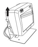
Lift the scanner straight up and out of its mount.
