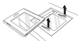
Lift off the Top Cover, then use the Lift Handles to remove the scanner from the counter.
