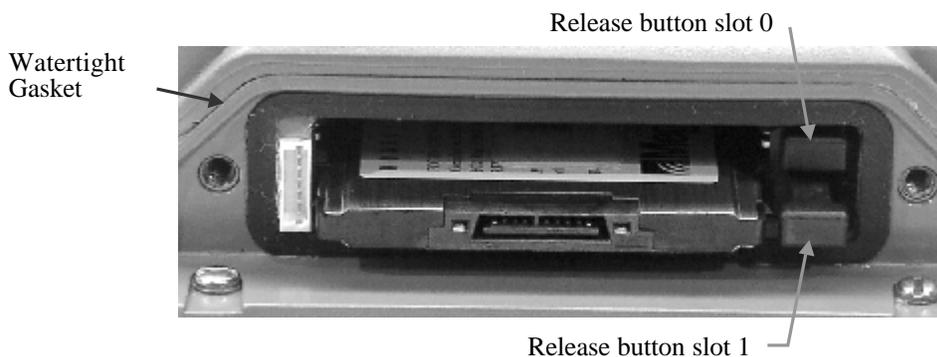
1. It is normally not necessary to turn off the CE5000 before inserting, removing or swapping a PC Card. This can be done any time while the unit is running or turned off.
