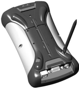
Using a screwdriver or the flat head of the stylus, lock the PowerBoot latches by turning them clockwise one half turn until the arrows on the latches point away from the I/O ports.
