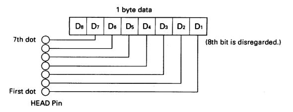
As will be understood from the above, the data are used in which the first dot corresponds to the first bit and the 7<sup>th</sup> dot corresponds to the 7<sup>th</sup> bit. The 8<sup>th</sup> bit is disregarded. Try to select decimal data or hexadecimal data matching to the host computer.
