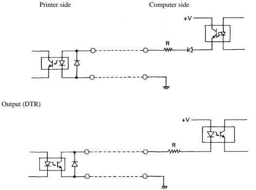
Note: Resistance should be set so that Current Loop is restricted within 10 ~ 20 mA.
