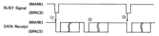
Double buffer transfer is made as follows.
