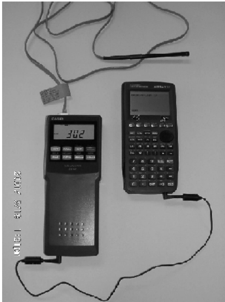
The Casio EA-100 Data Collector connected to the Casio FX2.0 Graphing Calculator
