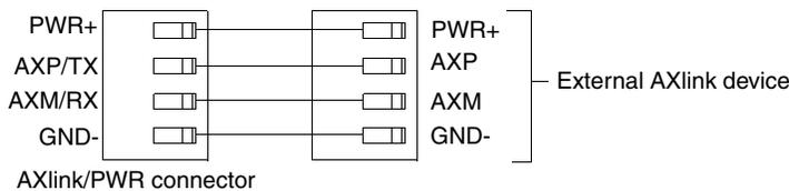
**FIG. 5** AXlink/PWR data and power wiring diagram
