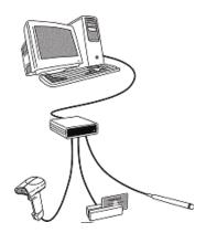
**NOTE: DO NOT USE USB EXTENSION CABLES** with the M2800. The USB standard was designed for keyboard cables with a length of 3 meters maximum. Use of a long USB extension cable may cause improper operation. If extra cable length is needed, the use of a USB hub device is required.
