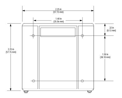
Mounting holes are threaded for four #6-32 screws.
