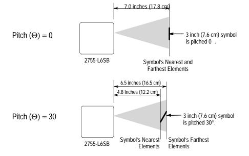
**Step 1 + Step 2.** With both of these aspects working together, the Read Range is shorter with a pitched symbol than with one that is not pitched. This results in:
