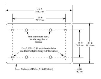
Figure 4.3 Installing With the Mounting Plate
