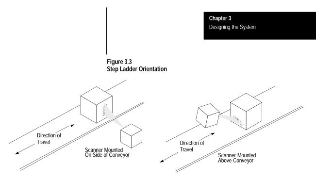
In general, **ladder orientation** (Figure 3.3) is preferred, because each scan covers a slightly different part of the symbol. This means that:
