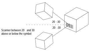
When using "A" range scanners to read symbols with high paper noise, increasing the skew to  $30^{\circ}$  may enhance performance.
