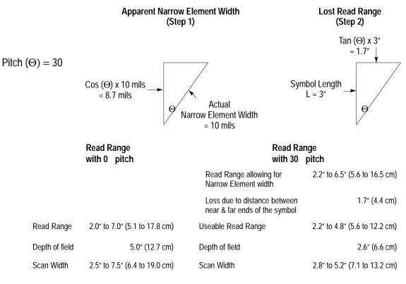
In picket fence orientation, the scanner and symbol are set as far apart as possible within the Read Range, to give the greatest number of scans per symbol. However with pitched symbols, the range is so narrow that the symbol is often placed in the center of the depth of field, where it is less apt to exceed the Read Range limits in either direction.
