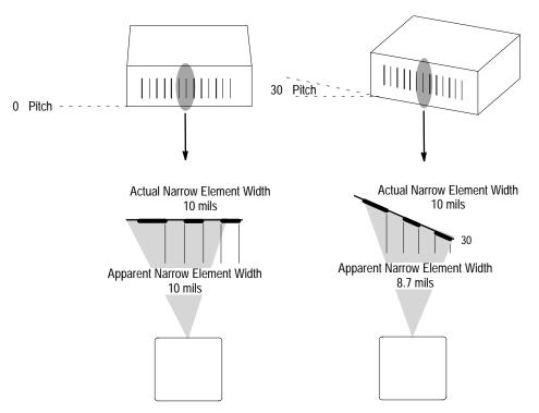
The *apparent* Narrow Element width is approximately the Cosine of the pitch angle, multiplied by the *actual* Narrow Element width. From Table 3.C,  $\cos(30)$  is 0.866.
