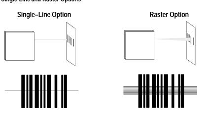
The raster type scanner is useful for reading poor quality bar code symbols. See Chapter 3 for application details.
