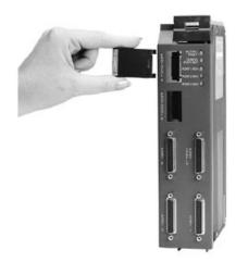
The Flexible Interface Module (cat. no. 2760-RB) is a two-slot module compatible with 1771-I/O chassis. The module has three interface ports for intelligent devices and one configuration port for menu-driven setup and diagnostics.
