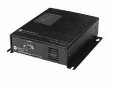
The Multi-Purpose Bar Code Workstation (cat. no. 2755-DH1) supports Allen-Bradley attended scanning devices and unattended versions of 2755-LD1 and -LD2. Use the workstation to decode and send scanned data to RS-232 or RS-422 host devices.
