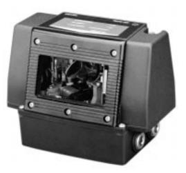
The AdaptaScan<sup>™</sup> Bar Code Reader combines an adjustable scanner and decoder in a compact NEMA Type 4 enclosure. The AdaptaScan Reader supports linear and raster scanning. Point-to-point and network communication options let the reader communicate with a variety of devices and networks.
