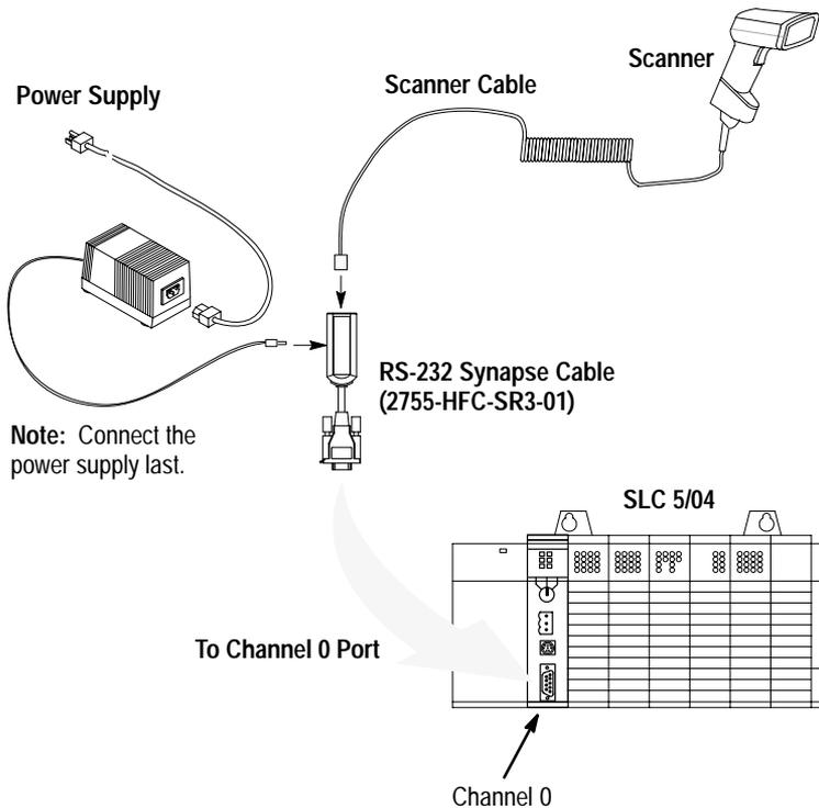
Refer to the user manuals for the Allen-Bradley Advanced Programming Software (APS) to make sure the Channel 0 settings match the Synapse cable settings.
