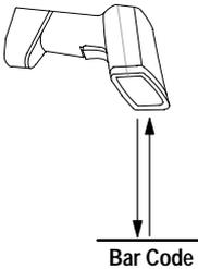
1. Specular reflection; reflected beam interferes.
