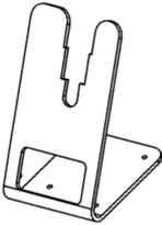
**Multi-mount Stand** – Rubber coated, fixed mount holder for counter or wall mounting.
