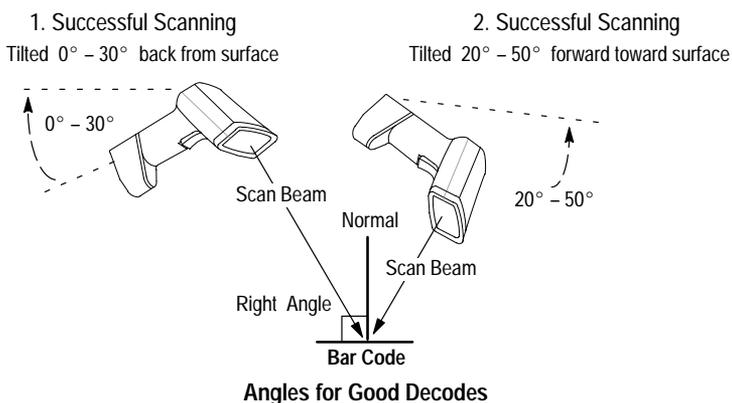
You can also scan successfully by tilting the scanner forward from parallel about  $20^\circ$  to  $50^\circ$  toward the scanning surface.
