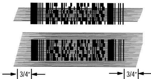
Scan Pattern Spreading over PDF417 Bar Code
