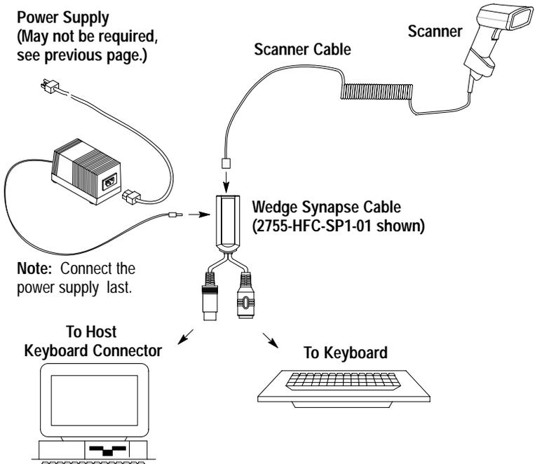
To connect the scanner cable to the keyboard wedge cable, push the cable into the connector until you hear the connector snap in place. To remove the scanner cable, press down on the small raised bump on the connector end and remove cable.
