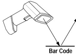
2. No specular reflection. Decode can occur.
