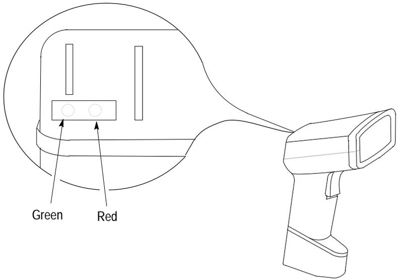
**Green LED = Decode**, indicating that a bar code symbol has been scanned and decoded. LED remains on until the next scan (trigger pressed).
