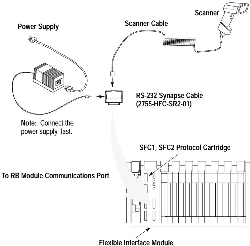
Refer to the user manual for the Flexible Interface Module for the proper configuration. Make sure the Synapse cable communications settings match the Flexible Interface Module settings for the port.
