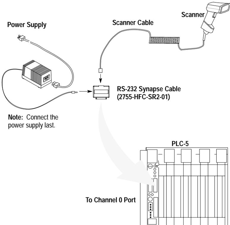
Refer to the user manuals for the Allen-Bradley 6200 Series Programming Software to make sure the Channel 0 settings match the Synapse cable settings.
