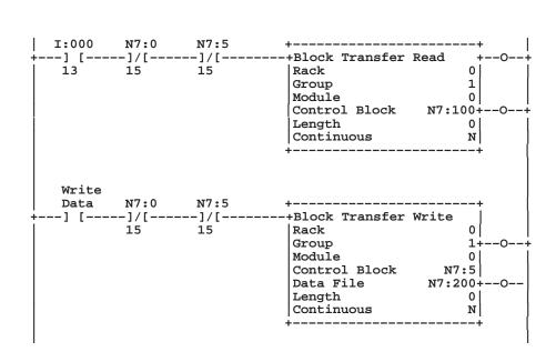
Figure 4 Sample PLC Program PLC 5/15/25 Etc. to 2760-RB
