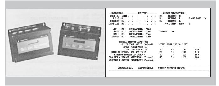
**Overview.** The Single and Dual-Head family of bar code decoders now support the Pharma-Code symbology as an option increasing their decoding capabilities in pharmaceutical product verification applications. The Pharma-Code enhancement is available by ordering Catalog No. 2755-DS1P, -DS4P, -DD1P, or -DD4P. The P in each catalog number denotes the additional capability to decode Pharma-Code symbols.
