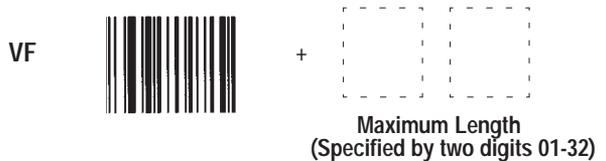
For example, to enter a maximum length of 05, scan the **VF** label, then scan codes 0 and 5 in Appendix B.
