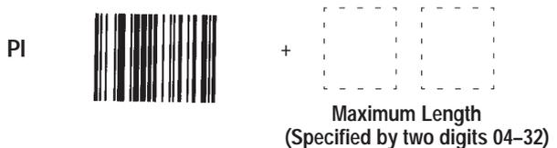
**If the minimum and maximum lengths are set equal, only codes of that exact length are read.**
