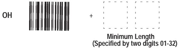
For example, to enter a minimum length of 05, scan the **OH** label, then scan codes 0 and 5 in Appendix B.
