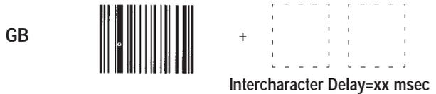
For example, to set the delay to 15 milliseconds, scan the **GB** label, then scan codes 1 and 5 in Appendix B.
