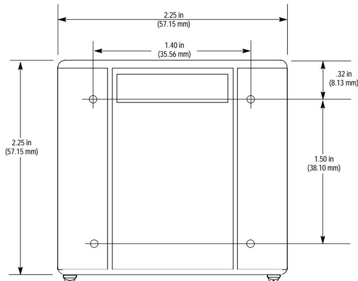
Mounting holes are threaded for four #6-32 screws.
