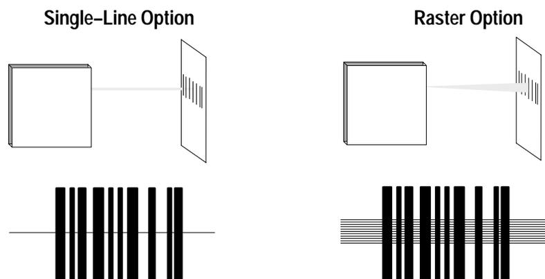
The raster type scanner is useful for reading poor quality bar code symbols. See Chapter 3 for application details.
