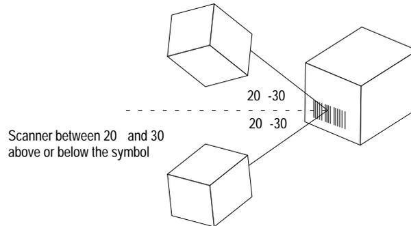
When using “A” range scanners to read symbols with high paper noise, increasing the skew to 30° may enhance performance.
