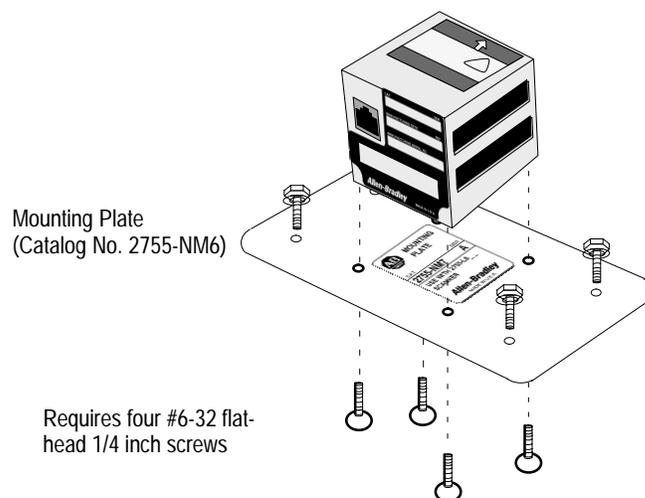
**Note:** The scanner has four threaded holes for mounting screws.
