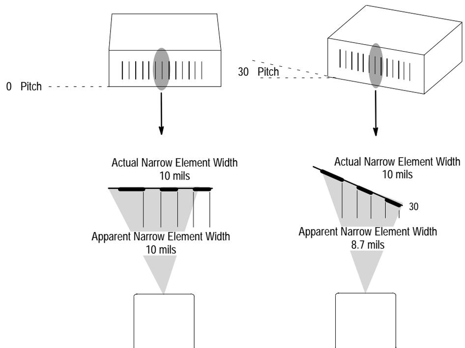
The *apparent* Narrow Element width is approximately the Cosine of the pitch angle, multiplied by the *actual* Narrow Element width. From Table 3.C,  $\cos(30^\circ)$  is 0.866.
