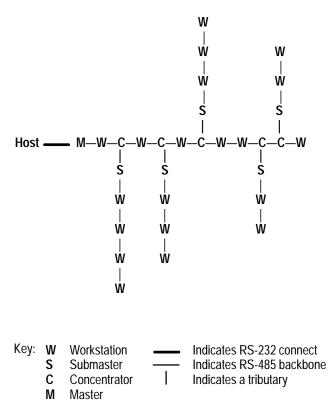
A workstation which is being used as a Master, Concentrator or Submaster can perform data collection functions even while serving in the communications network.
