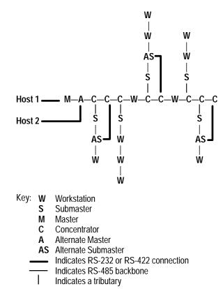
An Alternate Submaster will allow the communication operations to continue through a secondary Concentrator if the primary Concentrator becomes inoperable or is removed from the network.
