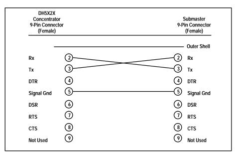
Figure D. 7 RS-422 Workstation/Any Host Connector
