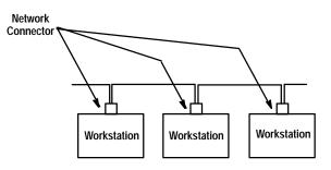
Figure 2.3 shows the correct method of wiring a network. This figure shows the cable coming into the Network Connector (Catalog No. 2708-NNC) and making connection with the cable coming out of the connector. If the workstations are removed from their respective network connectors, it is easy to determine that a continuous cable or bus has been created.
