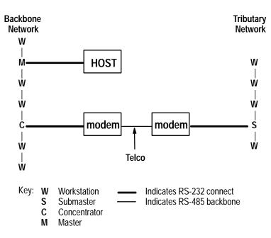
The extension of a network across telephone lines consists of placing a modem on one side of the line to connect with the Concentrator, and placing the other modem on the other side to connect with the Submaster.
