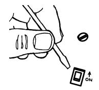
**Note:** The terminator switch should be OFF on all workstations except the MASTER and SUBMASTER. If other terminator switches are on, indeterminate network conditions will occur.
