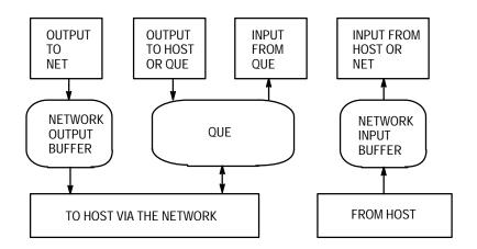
This diagram shows the various methods which can be used to move data into and out of a workstation through its network.
