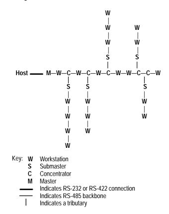
All of the workstations, including Masters, Concentrators and Submasters, are standard workstations which have been configured for their individual roles in the network. A configuration parameter is changed to allow any workstation to adopt a new role in the network. Each workstation is capable of operating in both a data collection and a data communications mode.
