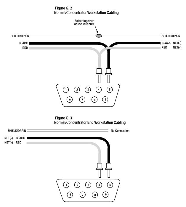
The previous network diagrams are for use in installations where the Network Connector (Catalog No. 2708-NNC) is not used. To fully understand the correct network wiring, it is **highly recommended** that Chapter 2 be carefully read.
