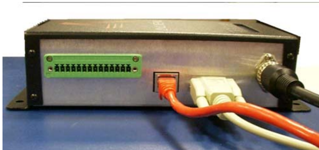
Figure 12 - RS-232, LAN, and Power Connections
