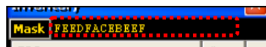
Masks defined with the EPC Prefix method are displayed on the utility screens as that initial part of the EPC.
