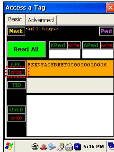
Pressing the red “write” buttons cause the reader to write the shown data in the field before writing it to the tag. The field turns orange while writing, and then turns white or red, depending on the success of the write operation.
