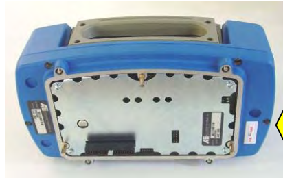
AXIOM Scan Head Shock Indicator Location
