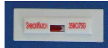
BAD Indicator (excessive shock, DO NOT install!)
