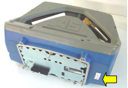
AXIOM-X Scan Head Shock Indicator Location
