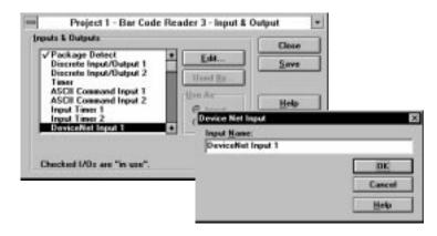
Each input can only be used once and inputs are only available for use by the Reader configuring the input. For example, if you configure a DeviceNet input for Bar Code Reader 2, you will only be able to use DeviceNet inputs from Bar Code Reader 2. Once selected, an input will not be available for use by other configurations (appears greyed out on dialogs).
