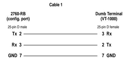
Cable 1 must be constructed to connect a configuration terminal to the 2760-RB module configuration port.
