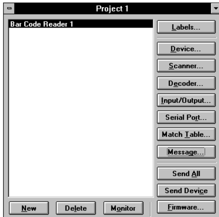
The Serial Port dialog defines communication parameters (RS-232/RS-485/RS-422) and protocols (ASCII, DH-485, DF1) for the reader's communication ports. Access it by selecting Serial Port in the Project dialog.
